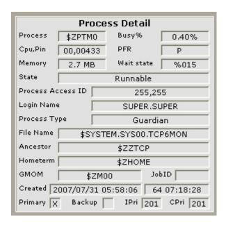
A right click on the CPU,PIN or Process field will bring up a menu allowing the User to select a variety of jumps or actions using the selected process (the actions available vary depending on the process):
