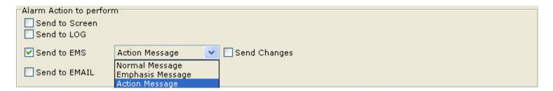
Email may be sent to either an individual address or a group. By default, only the first Alarm message is sent. The option "Send EMAIL when Alarm is Cleared" cause the Alarm clear to also be sent.
