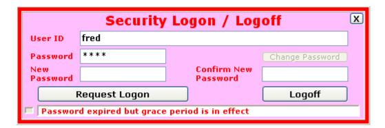
The MOMI server uses a password one time when the Request Logon button is pressed. A "logon server" process is created locked to an instance of the client. It is used to start additional MOMI server processes as needed to provide sensitive command processing for that instance of the client.
