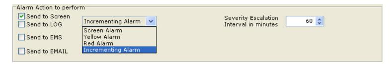
The MOMI LOG is an event file maintained by MOMI. It is accessed on the screen LogFile. Send Changes indicates that any change in the Alarm messages is logged. By default, only the first and last (or clear) are logged.
