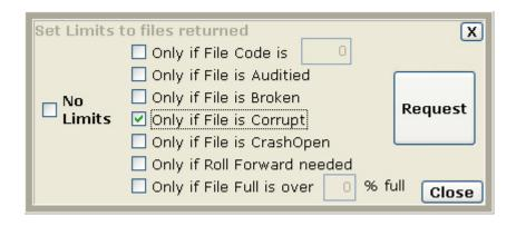
Files retrieved with Config limitation imposed attempt to optimize file retrieval for the fastest access. Only those records matching the criteria are returned to the Client. The above example requests only files with the Corrupt attribute. If multiple selections are made, these are 'and'ed' together (meaning everything checked must match).
